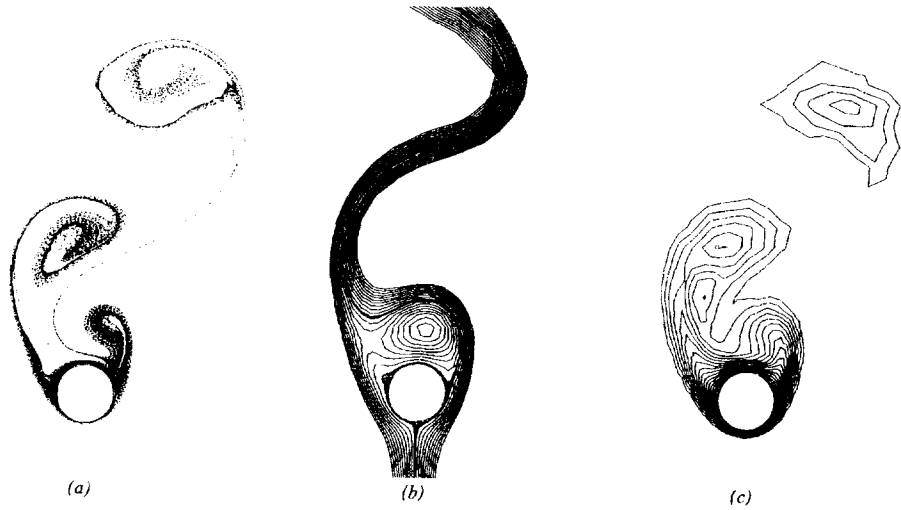
Figure 8. Numerical results of vortex shedding around cooled cylinder surface at Re = 100 ( Ri = -1.0 ): (a) streaklines; (b) streamlines; (c) isotherms
