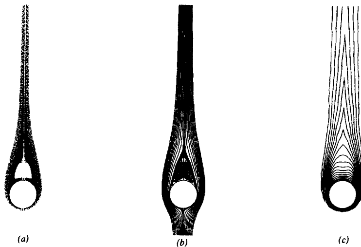
Figure 5. Numerical results of vortex shedding around heated cylinder surface at Re = 100 ( Ri = 0.5 ): (a) streaklines; (b) streamlines; (c) isotherms
